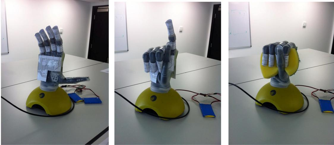
Figure 1: Prototype of Touch Bionics (iLimb) Sensorized prosthetic Hand with artificial Skin sleeve
